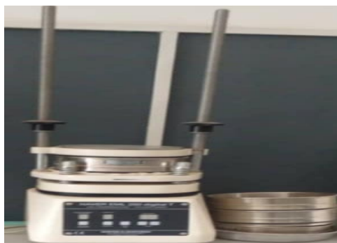
Figure 2. A 200 µm sieve (Haver EML 200 Digital T type).
