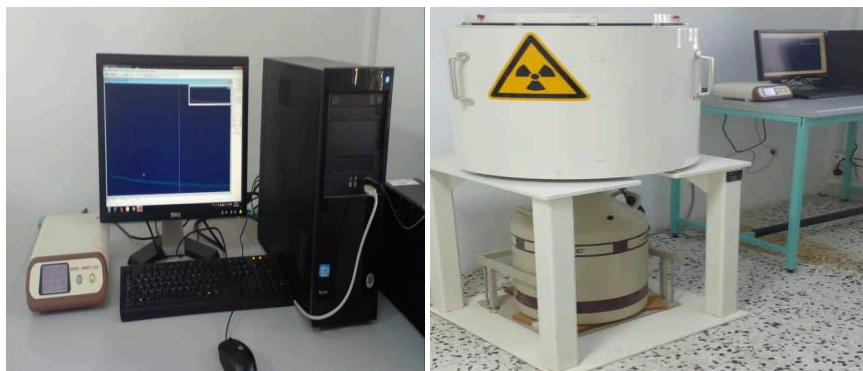
Figure 3. High-Purity Germanium (HPGe) gamma-ray spectrometry system used for measurements.
