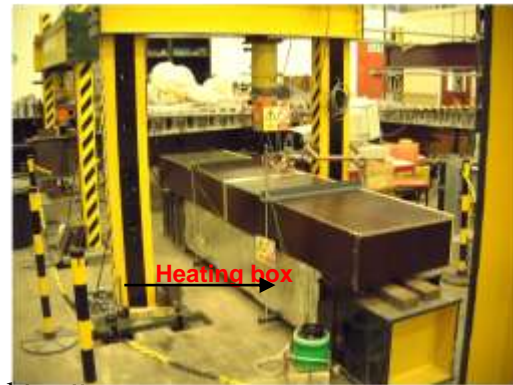
Figure 4 Thermal loading test set-up
